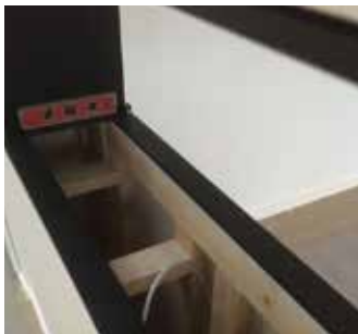
The hole for the burner is lined with wood.
